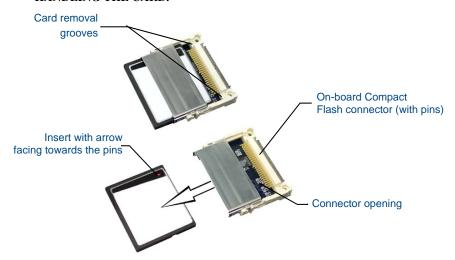
FIG. 7 Removing/installing a Compact Flash Memory card
